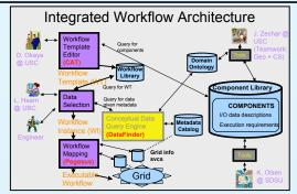
Architecture of the SCEC CME integrated workflow process. Workflow templates, which describe an abstract workflow, are instantiated to produce a concrete plan which can be executed on the computational grid. DataFinder's role in workflow instantiation is to locate already existing data files which would otherwise need to be computed.
