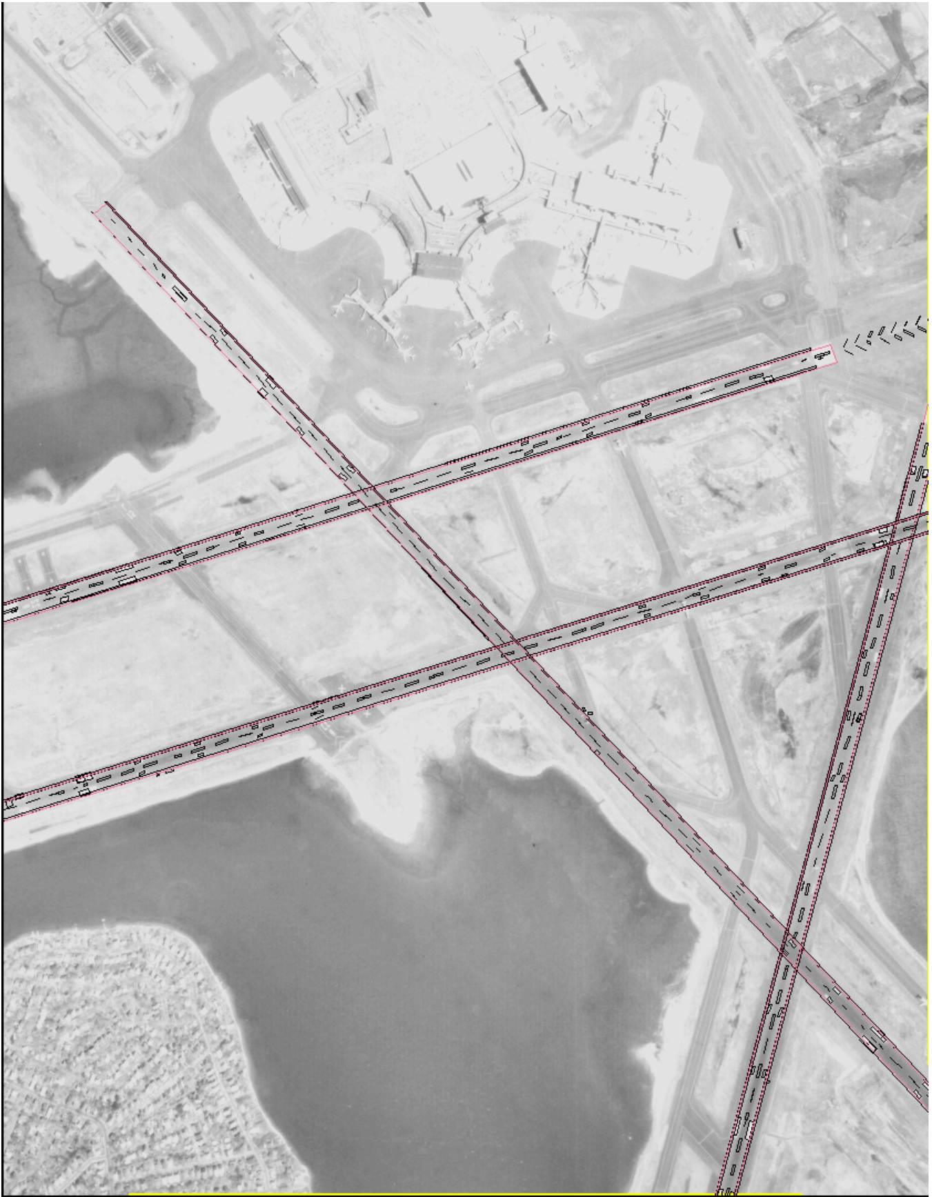
Figure 8 Boston Logan image with potential runways and their markings. The image has been brightened to make the markings display more visible.
