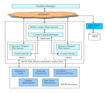
Fig. 6. New BDW system Architecture
