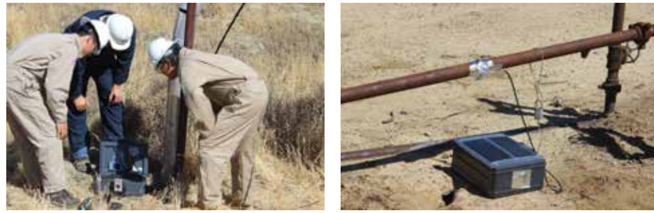
Deployed energy harvesting sensors for cold oil blockage detection research (CiSoft SEN)
