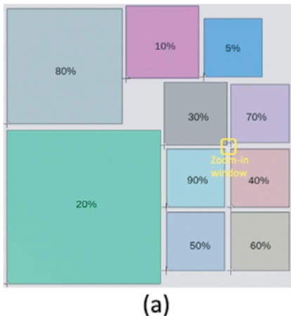
Figure 1. MPW chip placement flow optimizing density and density gradients between chips on the MPW reticle.
