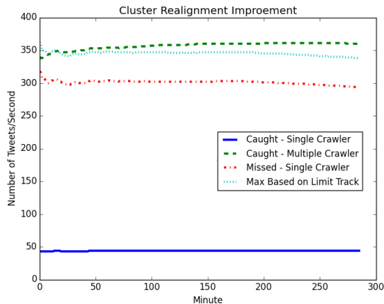
Figure 8: Performing cluster realignment by maintaining and updating the word co-occurrence graph over a long period of time can improve the number of tweets gathered per second without the need to introduce additional crawlers. Initially, the lack of a significant sample for the co-occurrence graph causes fluctuations in the gathering rate but as the sample size increases the volume of data per second becomes stable and is still able to maintain a constant rate of growth even as the amount of data in the population (limit maximum) reduces.
